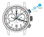
To stop the timing, press push-**button A** once more and read the 2 chronograph counters, for example: 10 mins/8 seconds.
