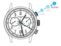
To restart the timing, press push-**button A** again (timing is resumed).
